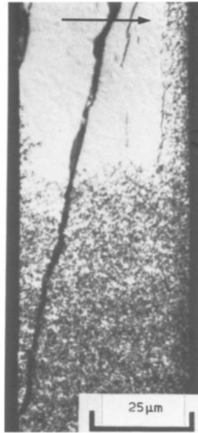
Figure 5 40 at% Mo ribbon showing both featureless substoichiometric \delta NiMo and regions of transformed microcrystalline structure. Arrow, growth direction.
